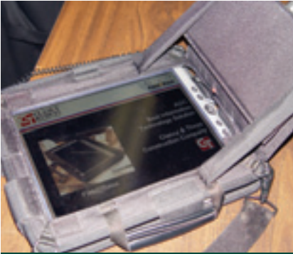
The F2B tablet PC has been designed for the rough environment of the job site. The tablet will run for two hours or more, depending on the type of battery pack.
